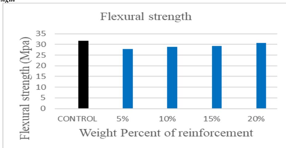
Figure 3: Impact of CCF on the Bending Strength of Recycled HDPE Composites
