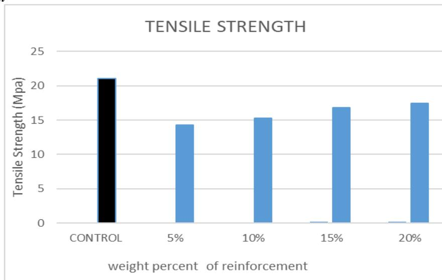
Figure 1: Impact of CCF on the Tensile Strength of Recycled HDPE Composites
