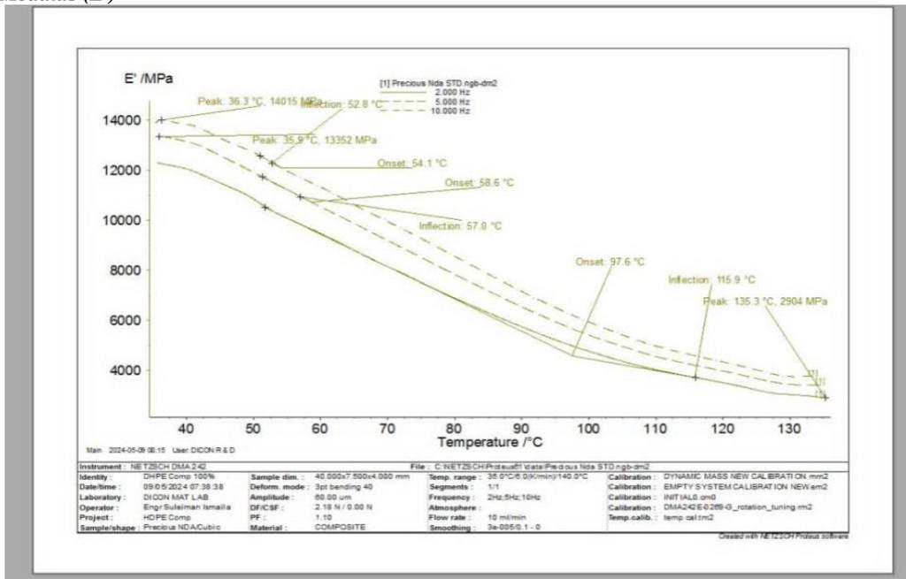
Figure 4: Storage modulus curve of waste HDPE composite at 2, 5, and 10 Hz
