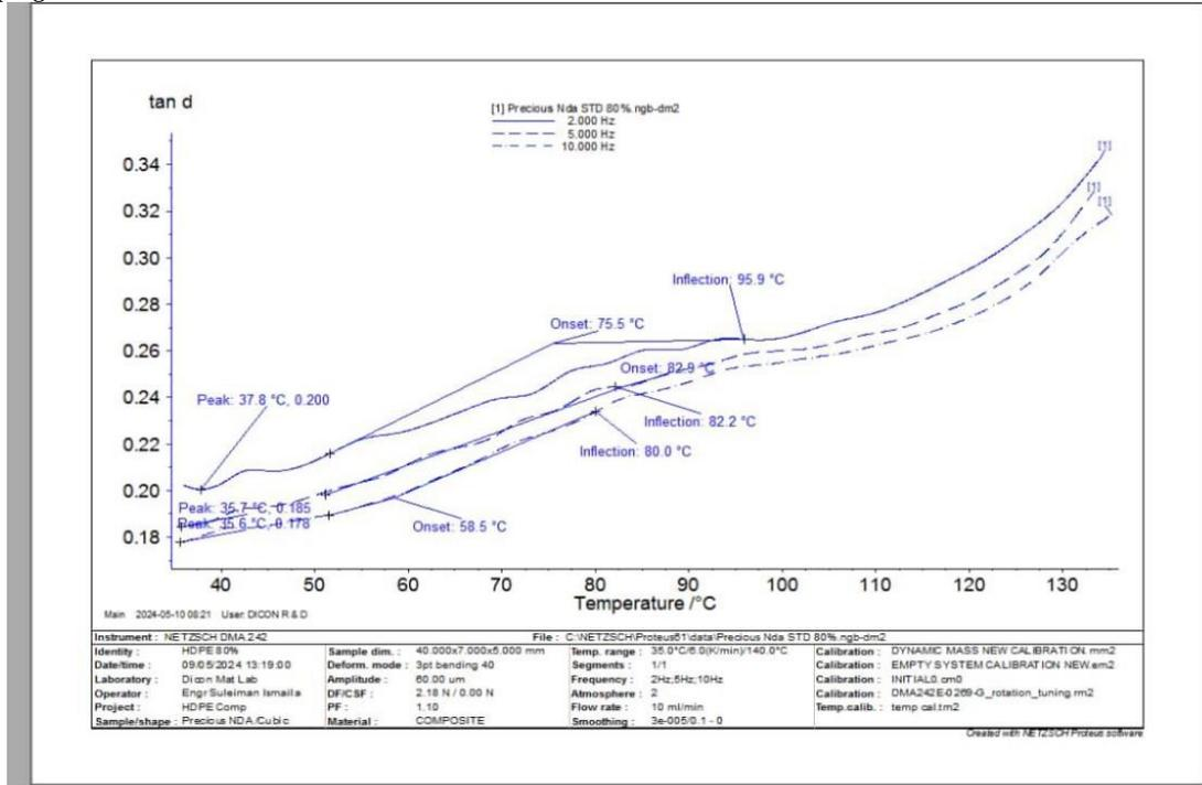
Figure 6: Damping curve of 80% waste HDPE and 20% CCF
