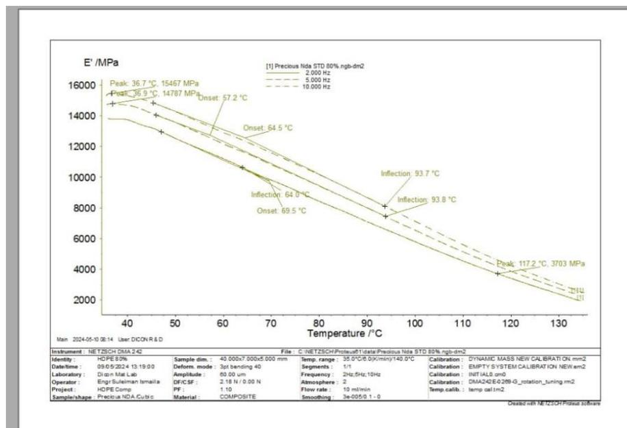
Figure 5: Storage modulus curve of waste HDPE and 20% CCF at 2, 5, and 10 Hz
