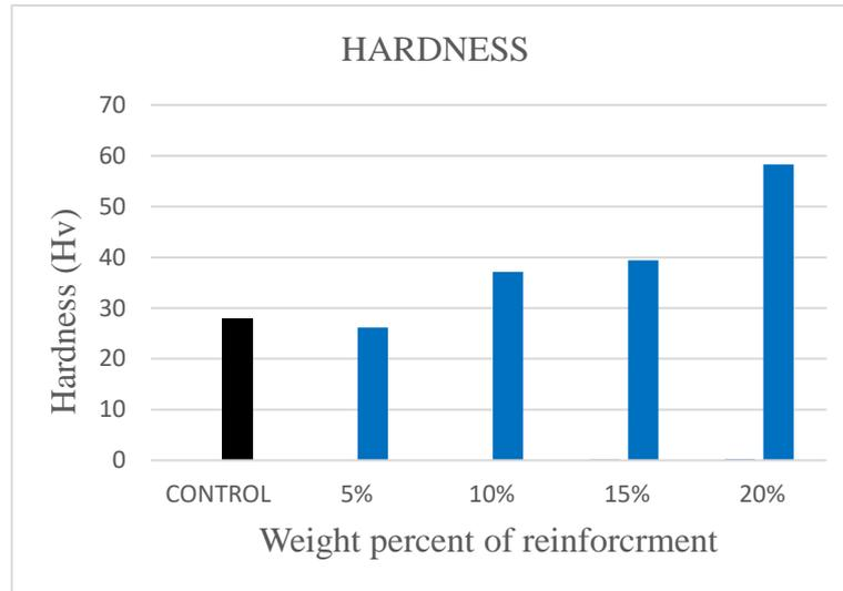
Figure 2: Impact of CCF on the Hardness of Recycled HDPE Composite
