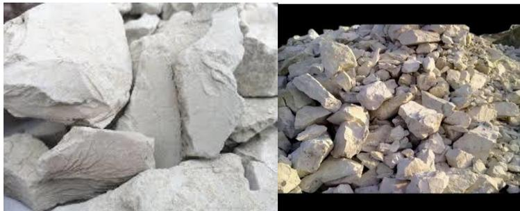
Figure 2: Lokoja Sodium Bentonite clay
