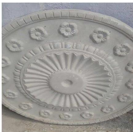
Figure 5: Moulded plaster of Paris produced using casting and pushing methods
