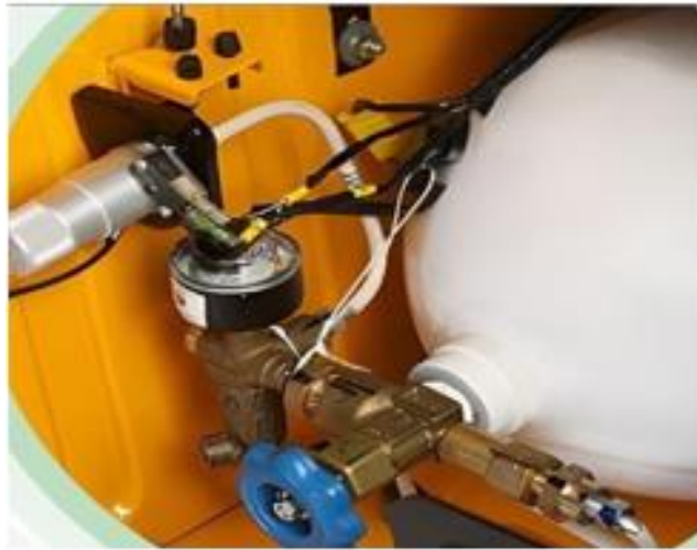
Figure 4: Some typical safety features attached to CNG tank (Presidential Compressed Natural Gas Initiative, 2024)
