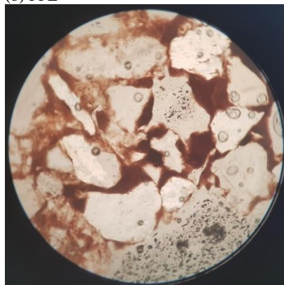
Plate 10: Photomicrographs of Massive Sandstone from Upper Bima Sandstone as observed under the microscope. Magnification x10
