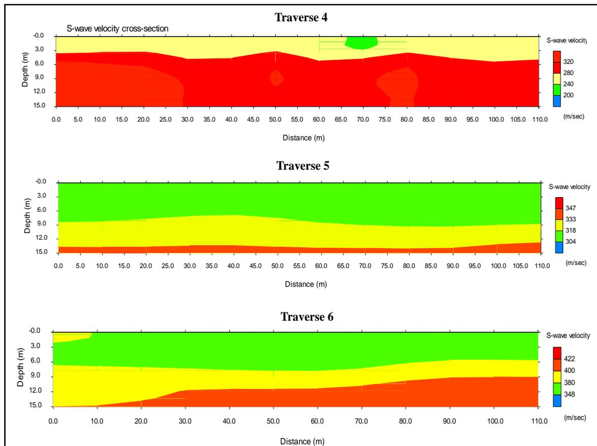
Figure 9: Shear wave velocity ( $V_s$ ) model for traverses 4 to 6. The shear wave velocity of the soil can be categorized into two, a relatively high  $V_s$  top layer (thickness ranging from 3 – 9 m), followed by a layer with higher  $V_s$ , indicating a stiffer material
