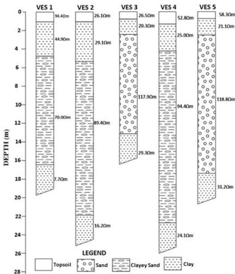
Figure 7: Geoelectric section showing the results obtained for VES 1 – 5
