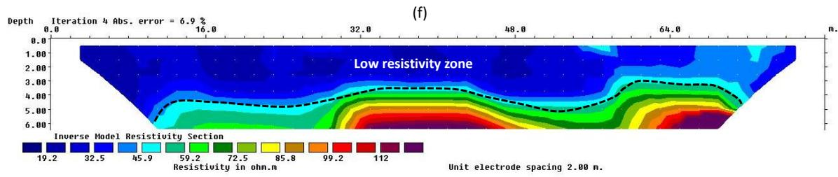
Figure 4: 2D Electrical resistivity along (a) Traverse 1 (b) Traverse 2 (c) Traverse 3 (d) Traverse 4 (e) Traverse 5 (f) Traverse 6. The topsoil is characterized by a low resistivity zone that can pose a threat to the stability of road pavement
