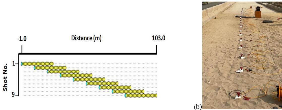
(a) Figure 2: (a) The schematic of the roll-along technique of the MASW measurements adopted in this study. In this case, for traverse 1. (b) The linear array arrangement of the geophones on the paved surface. Styrofoam was adopted to allow for contact between the ground and the geophone
