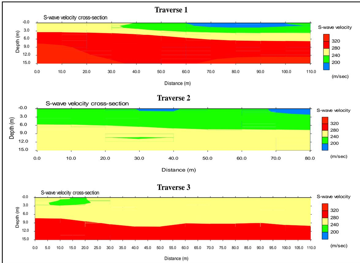
Figure 8: Shear wave velocity ( $V_s$ ) model for traverses 1 to 3. Low velocity lenses are observed on traverse 1 and 2
