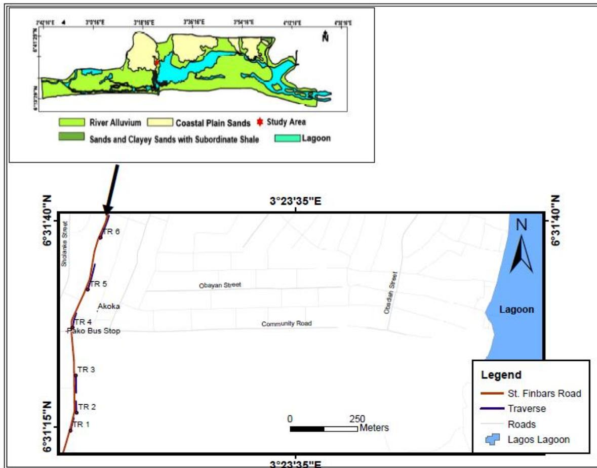
Figure 1: Geological map of Lagos showing the survey location and the basemap highlighting the ERT and MASW traverses
