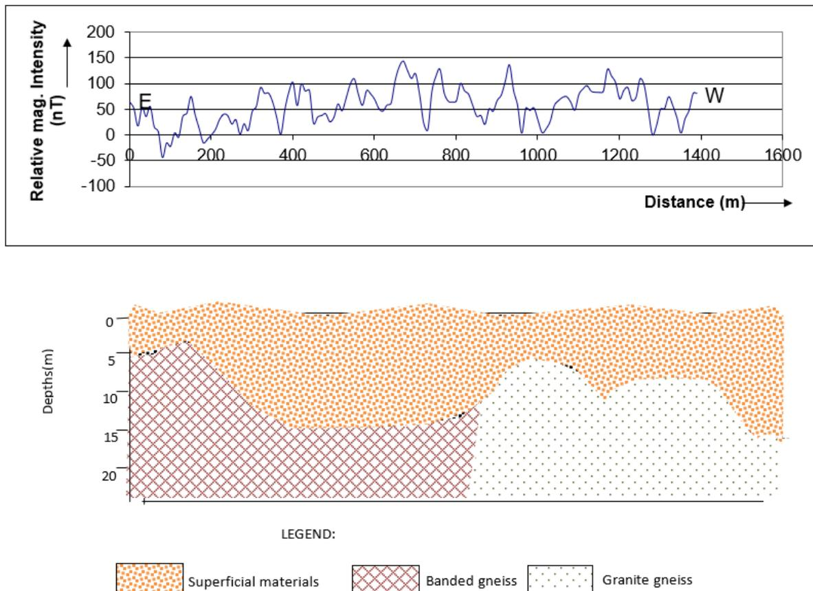
Figure 2: Total ground magnetic profile and its corresponding geomagnetic section along Traverse 1
