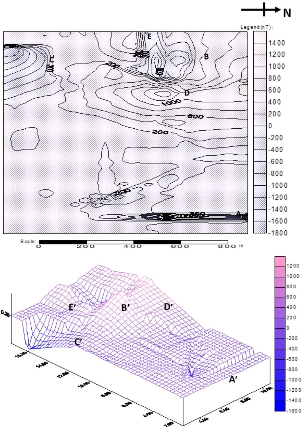
Figure 4(a): Ground magnetic contour map of the total field component (b) 3D Perspective view of the total field component
