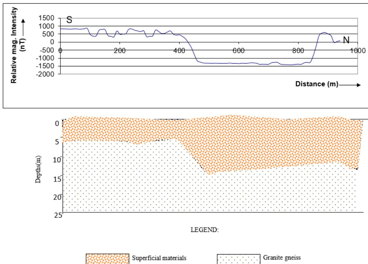
Figure 3: Total ground magnetic profile and its corresponding geomagnetic section along Traverse 10
