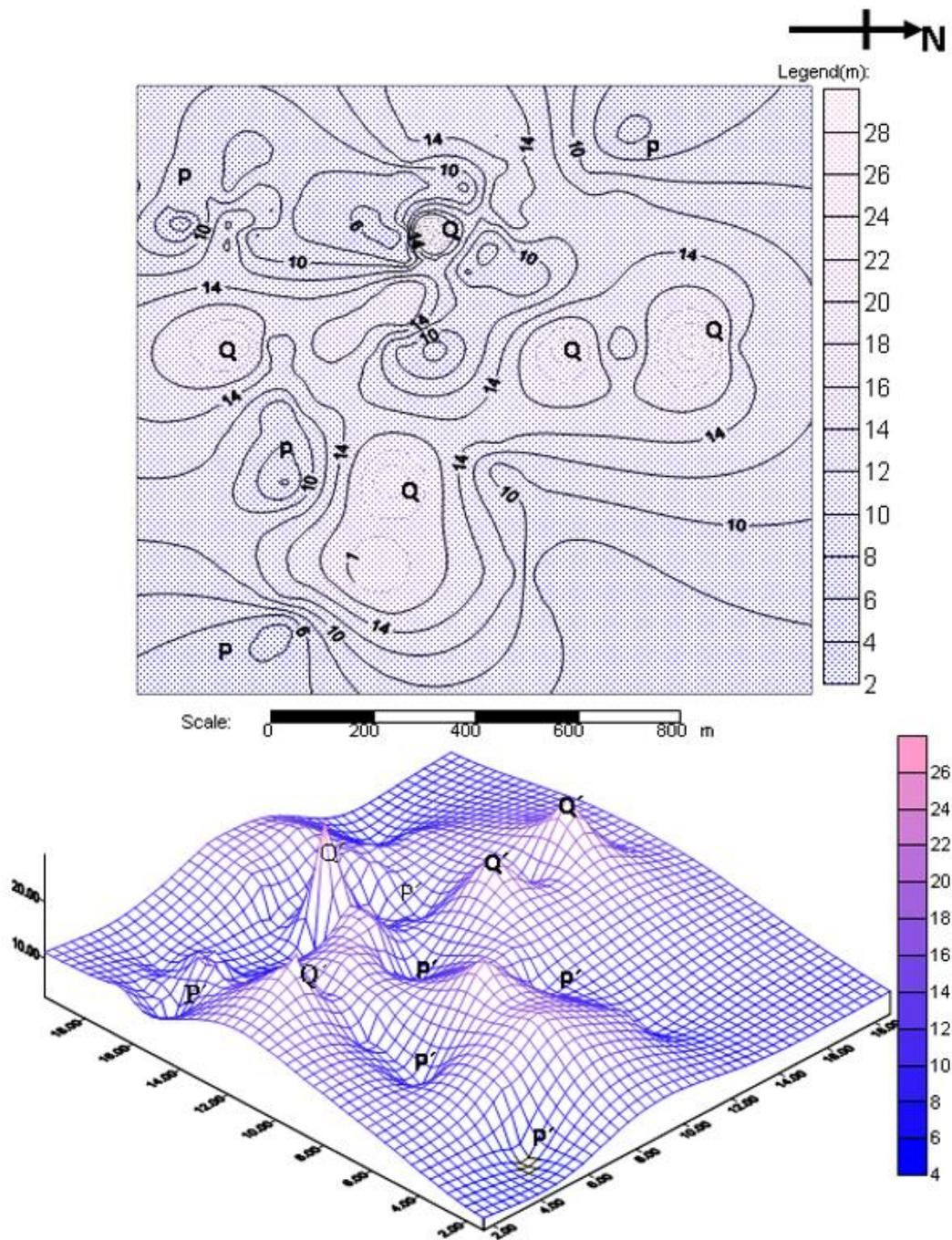
Figure 5 (a): Depth Distribution map of the study area from total field component (b) 3D Perspective view of the total field component
