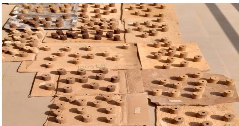
Figure 3: Sample of fuel briquettes produced from rice husk and palm kernel shell
