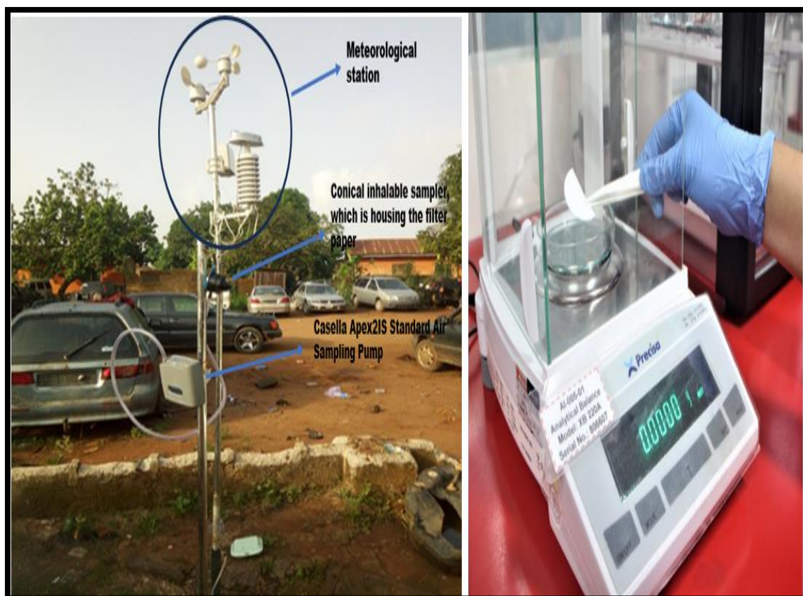
Figure 1: Set up for the collection of PM 2.5 , Meteorological parameters and the gravimetry determination of the weight of the filter paper (Onaiwu & Eferavware 2023; US EPA 2013; Onaiwu & Ifijen 2024).
