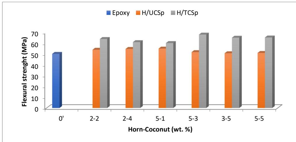
Figure 5b: Flexural strength of hybrid horn and untreated/treated coconut shell particles reinforced epoxy composites
