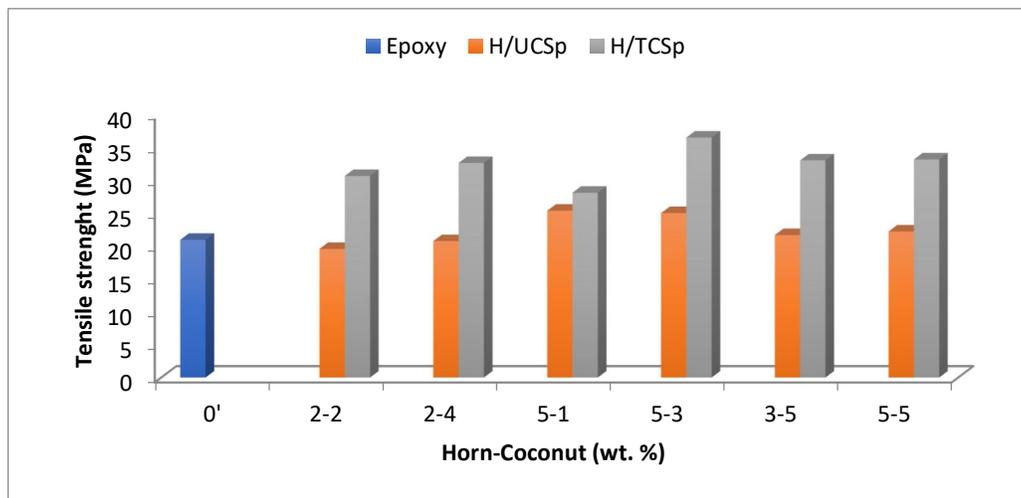
Figure 4b: Tensile strength of hybrid horn and untreated/treated coconut shell particles reinforced epoxy composite
