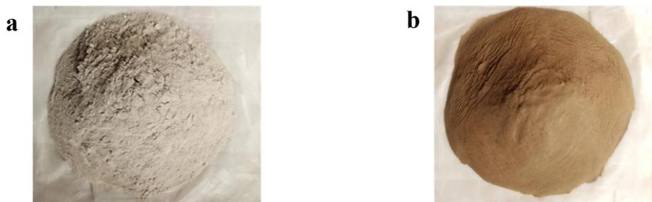
Figure 1: (a) sheep horn particles (b) coconut shell particles
