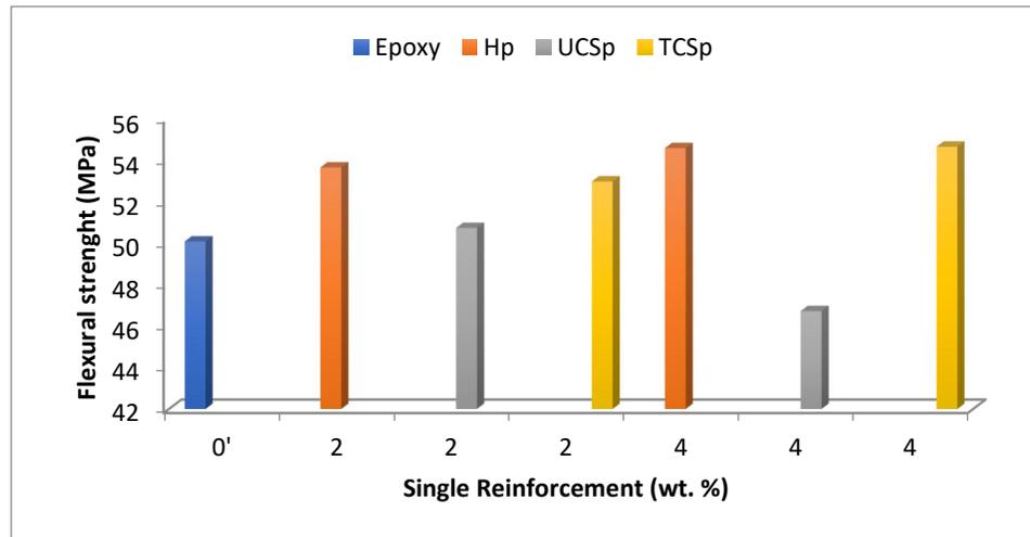
Figure 5a: Flexural strength of horn, untreated and treated coconut shell particles reinforced epoxy composites
