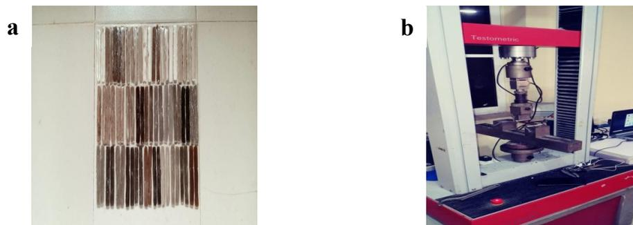
Figure 3: (a) Flexural test samples (b) Flexural test set-up
