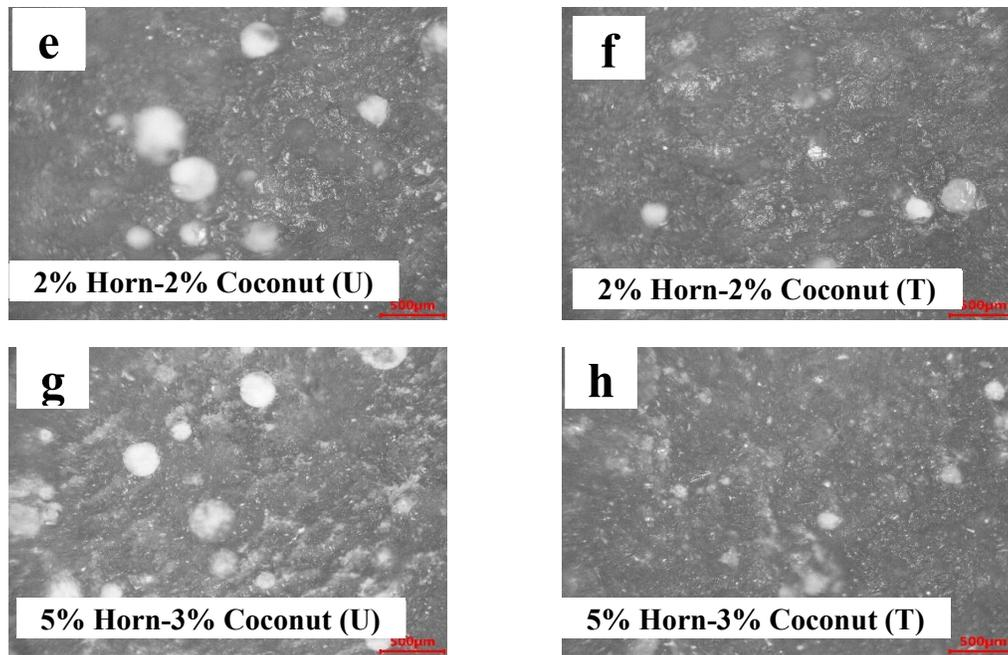
Figure 6: (a) Optical micrograph of pure epoxy, (b - d) Optical micrographs of the composite containing single reinforcement, (e - h) Optical micrographs of the hybrid composites
