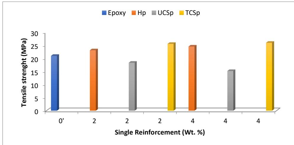
Figure 4a: Tensile strength of horn, untreated and treated coconut shell particles reinforced epoxy composite
