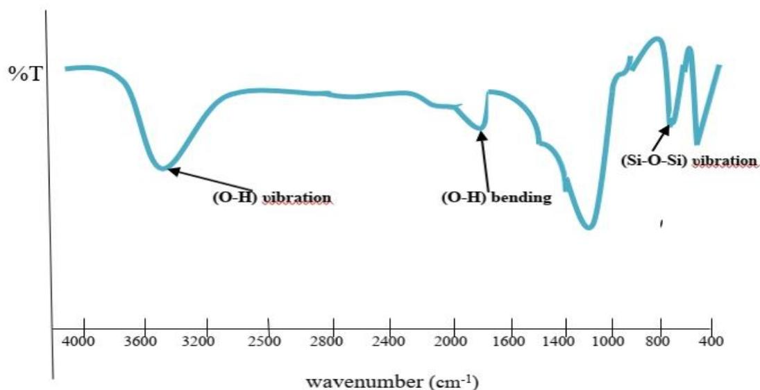
Figure 2: The FTIR spectra of the silica nanoparticles synthesized from sugarcane waste.
