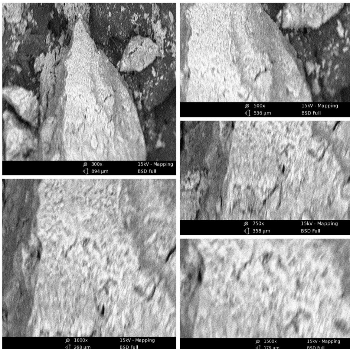
Figure 5: The SEM photograph of silica microparticles synthesized using extraction and precipitation method
