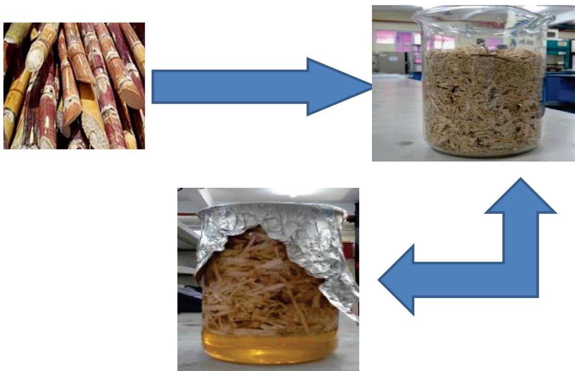
Figure 1: Treatment of Sugarcane Waste with Hcl to Remove Impurities
