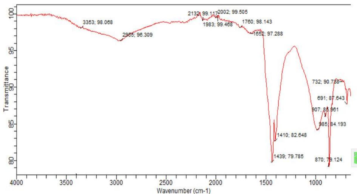
Figure 3: The FTIR spectra of silica microparticles synthesized from sugarcane waste
