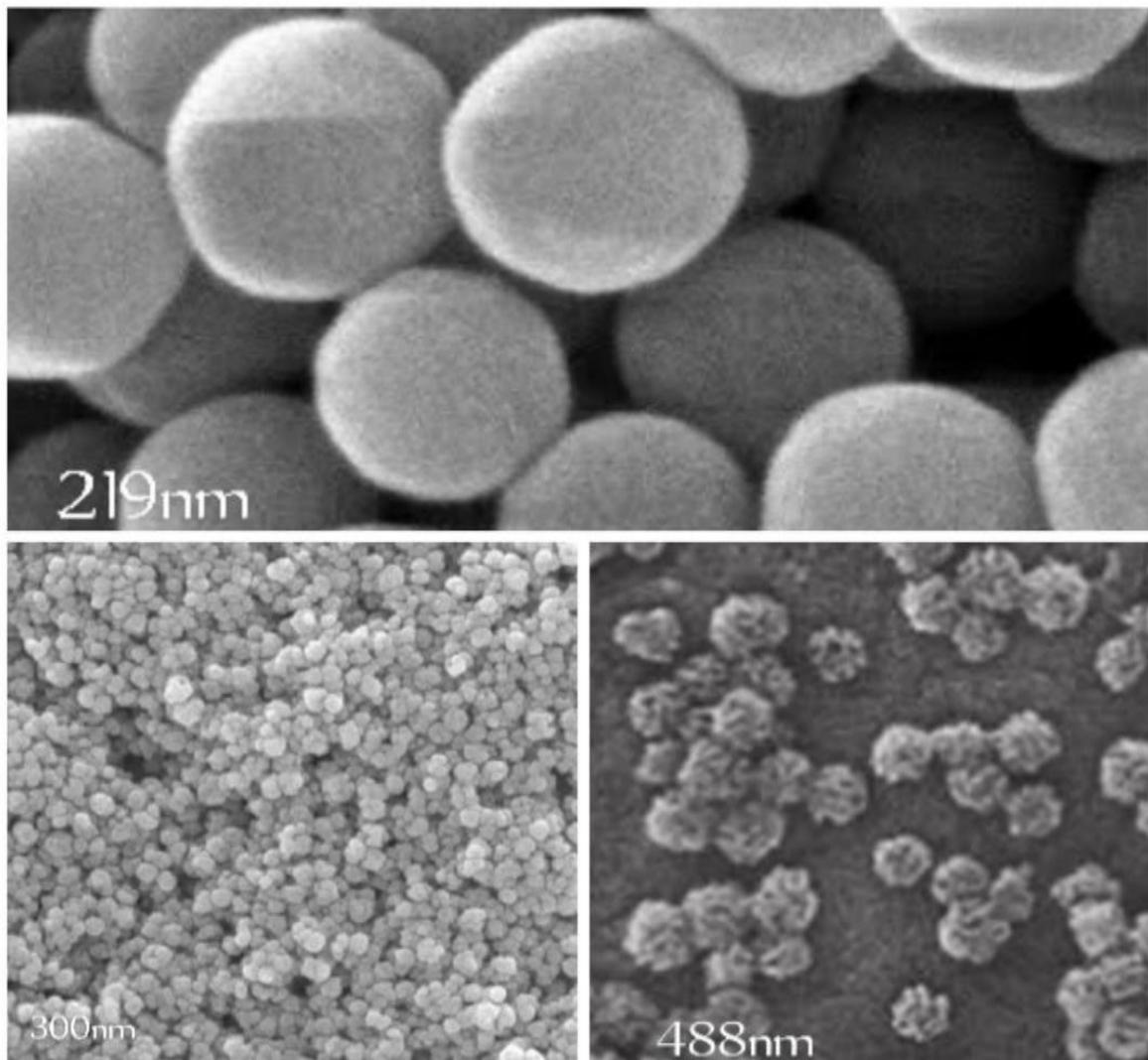
Figure 4: The SEM photograph of silica nanoparticles produced using extraction and precipitation method
