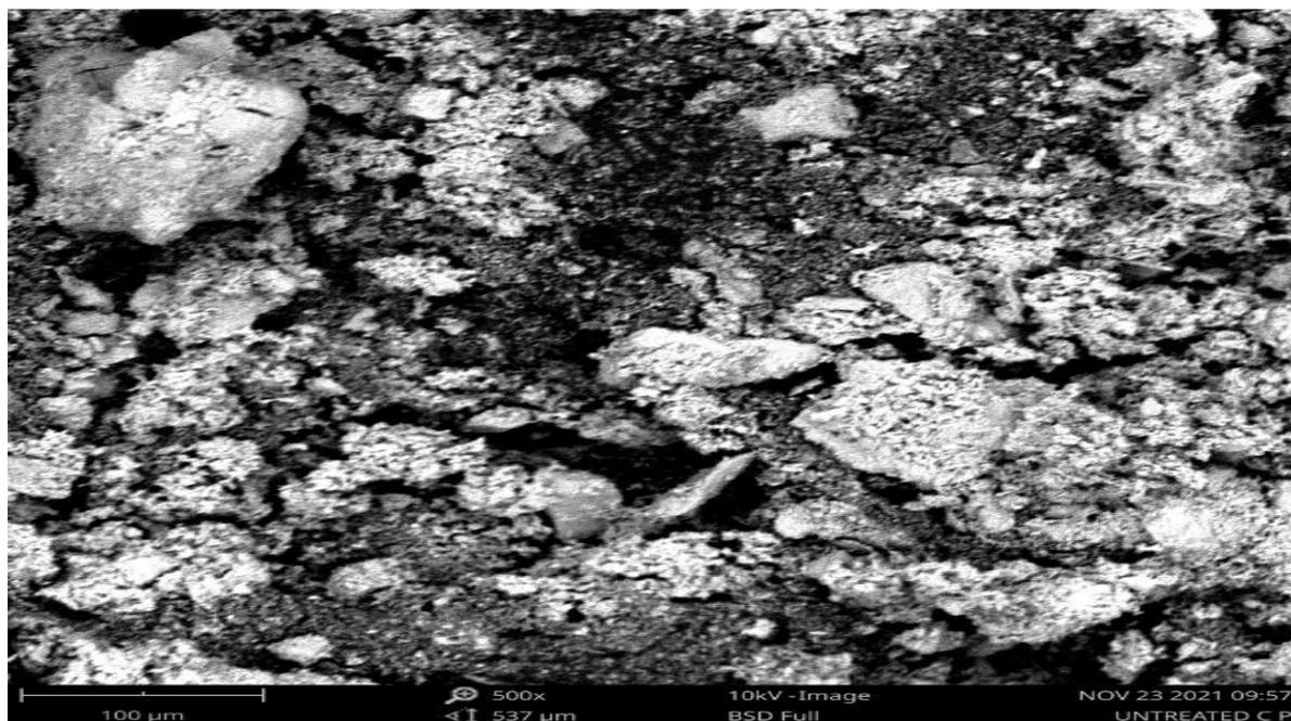
Plate 1: Untreated Cassava Peel SEM
