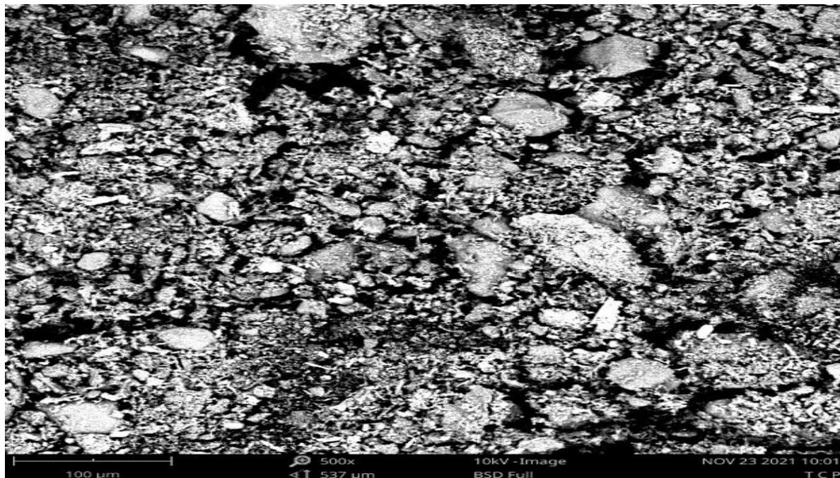
Plate 2: Treated Cassava Peel SEM
