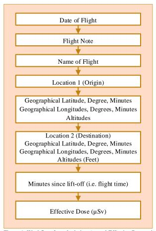
Figure 1: Workflow for calculating Annual Effective Dose using CARI 6M (Hwang et al. 2014)
