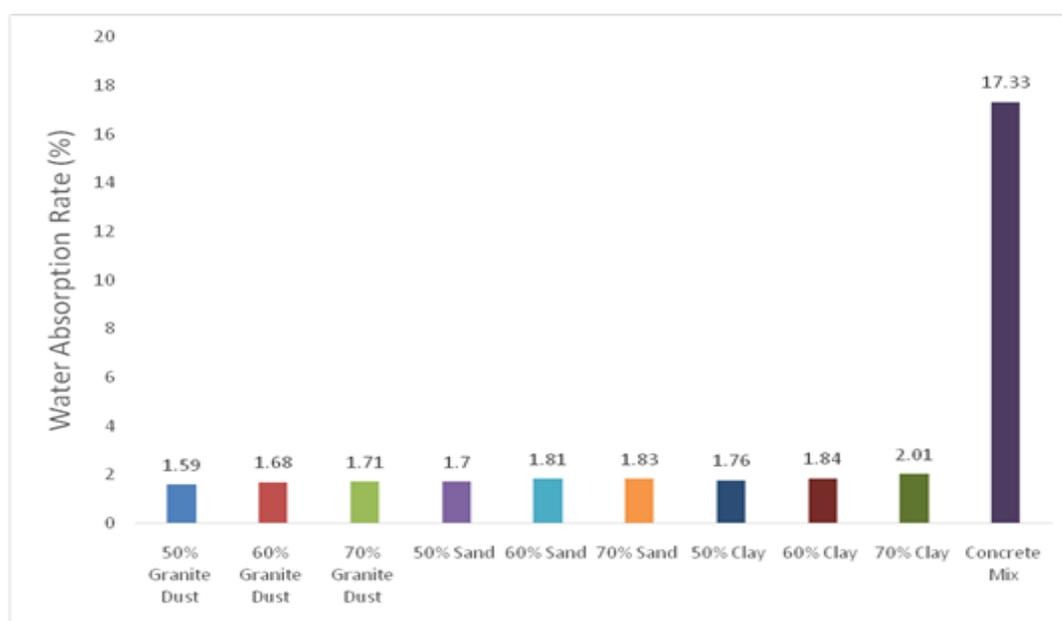
Figure 8: Comparison of pavers from varying ratio of plastic melts/geological materials and Cement pavers based on their water absorption rate.
