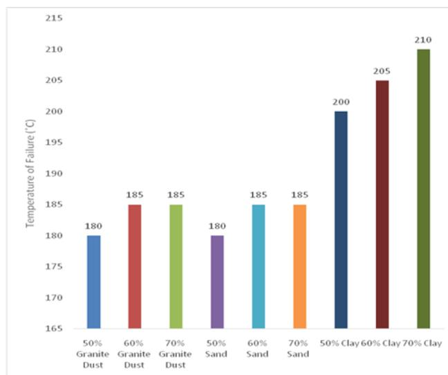
Figure 9: Comparison of failure temperatures of pavers from varying ratio of Plastic/geological materials
