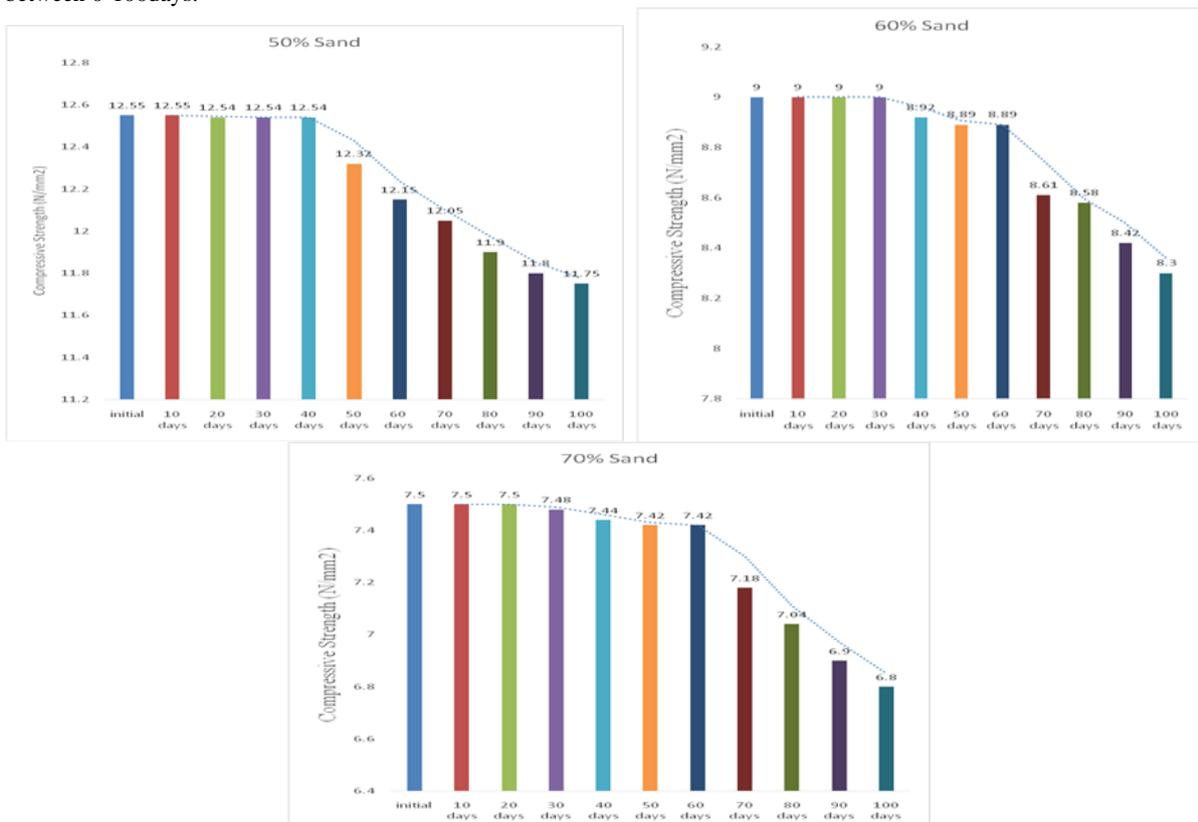
Figure 5 d-f: Chart of compressive strengths of pavers made of sand and plastic additives in different ratios a: Sand/Plastic=50/50, b: Sand/Plastic=60/40 and c: Sand/Plastic=70/30 on activation with weak sulphuric acid for between 0-100days.
