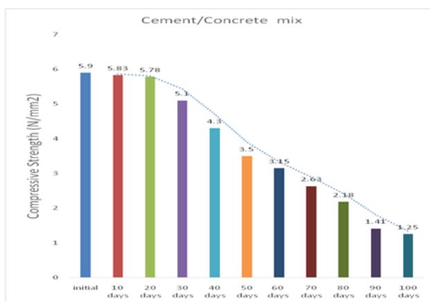
Figure 7 j: Chart of compressive strengths of pavers derived from cement on activation with weak sulphuric acid for between 0-100days
