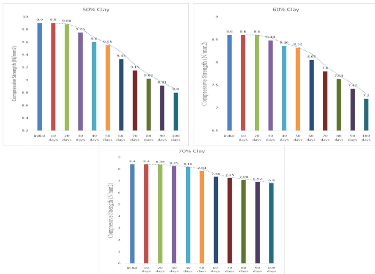
Figure 6 g-i: Chart of compressive strengths of pavers made of clay and plastic additives in different ratios a: Clay/Plastic=50/50, b: Clay/Plastic=60/40 and c: Clay/Plastic=70/30 on activation with weak sulphuric acid for between 0-100days.
