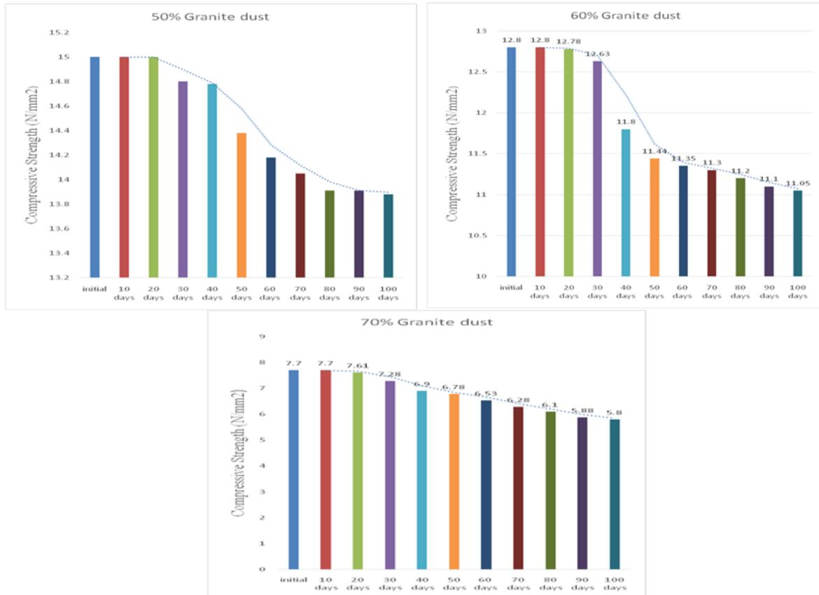
Figure 4 a-c: Chart of compressive strengths of pavers made of granite and plastic additives in different ratios a: Granite/Plastic=50/50, b: Granite/Plastic=60/40 and c: Granite/Plastic=70/30 on activation with weak sulphuric acid for between 0-100days.
