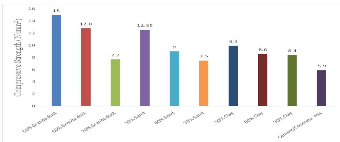
Figure 3: Comparison of pavers from varying ratio of plastic melts/geological materials and Cement pavers based on their compressive strength.
