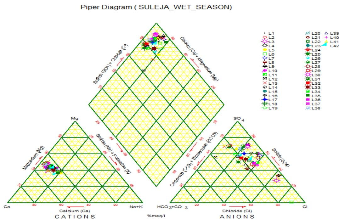
Figure 3: Hydrochemical Characterization of groundwater of Suleja Plotted on Piper Trilinear diagram for the wet season.
