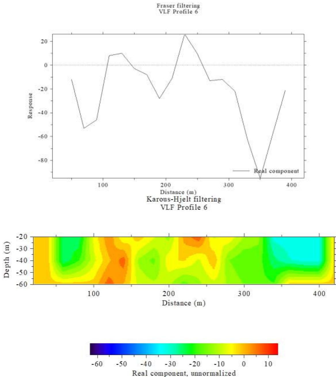
Figure 9: Current density distribution across VLF-EM Transverse 6
