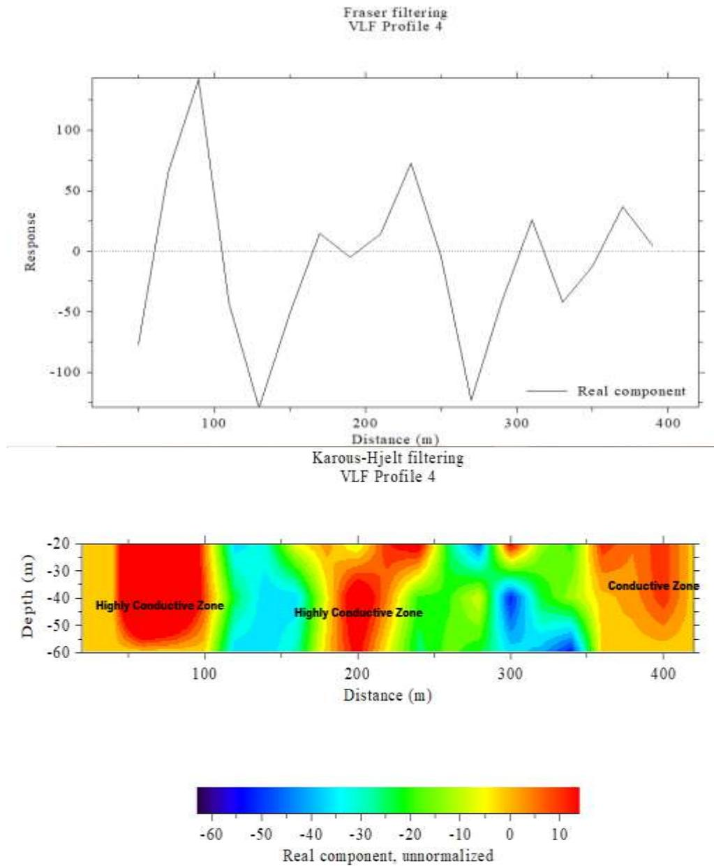
Figure 7: Current density distribution across VLF-EM Transverse 4
