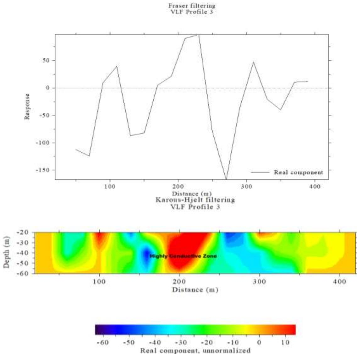
Figure 6: Current density distribution across VLF-EM Traverse 3
