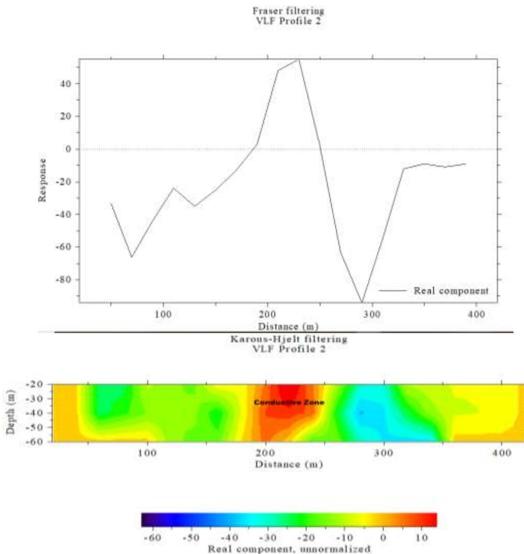
Figure 5: Current density distribution across VLF-EM Traverse 2
