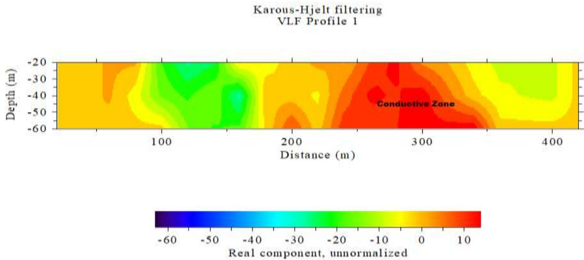
Figure 4: Current density distribution across VLF-EM Traverse 1
