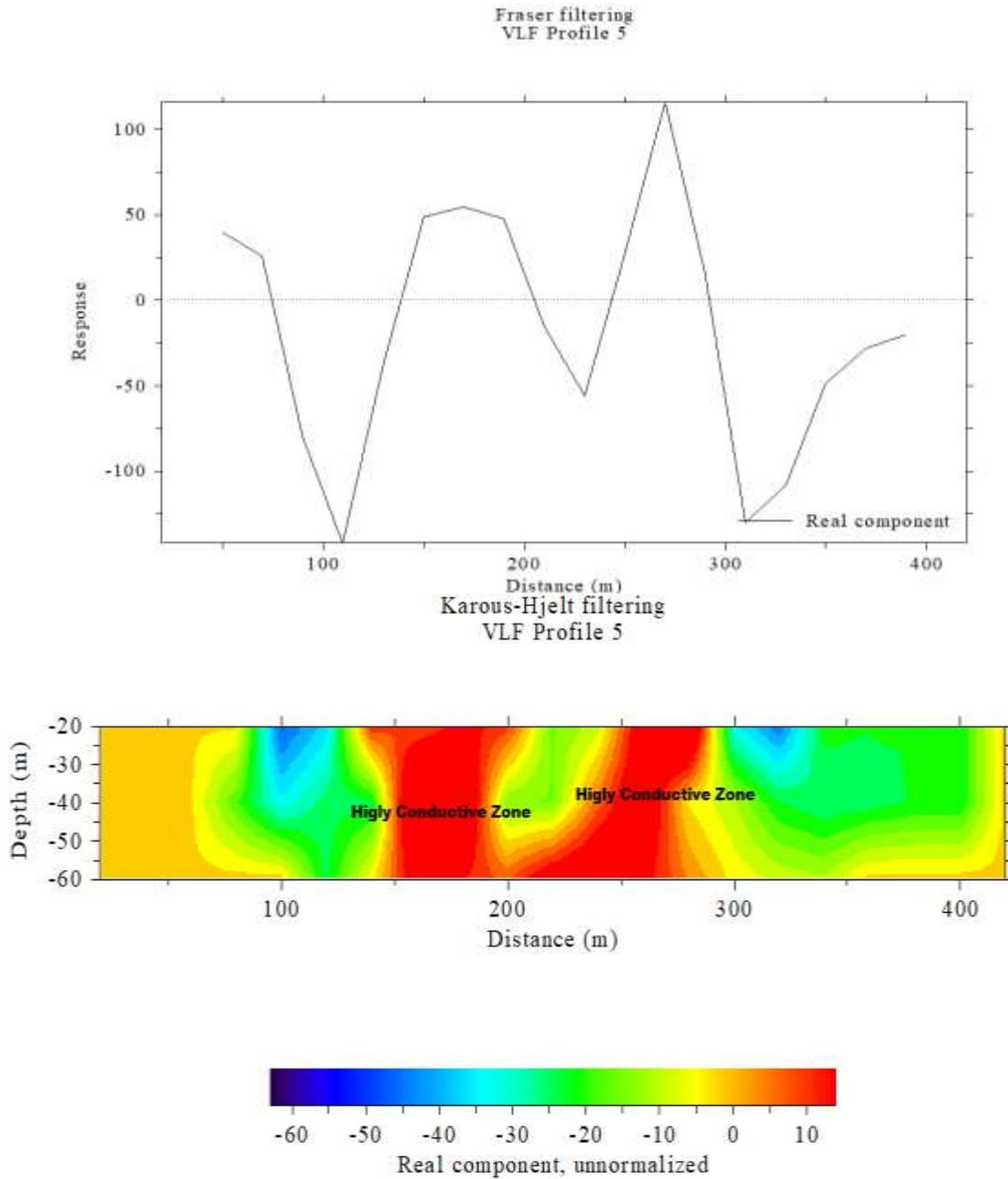
Figure 8: Current density distribution across VLF-EM Transverse 5
