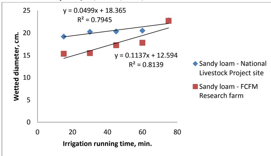
Fig. 2: Wetted diameter variation with irrigation running time
