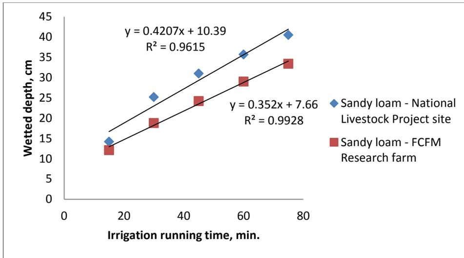
Fig. 3: Wetted depth variation with irrigation running time
