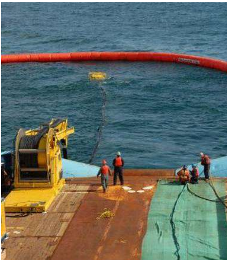
Fig. 2: Use of Boom and Skimmers (Source: Barnes, 2015)
