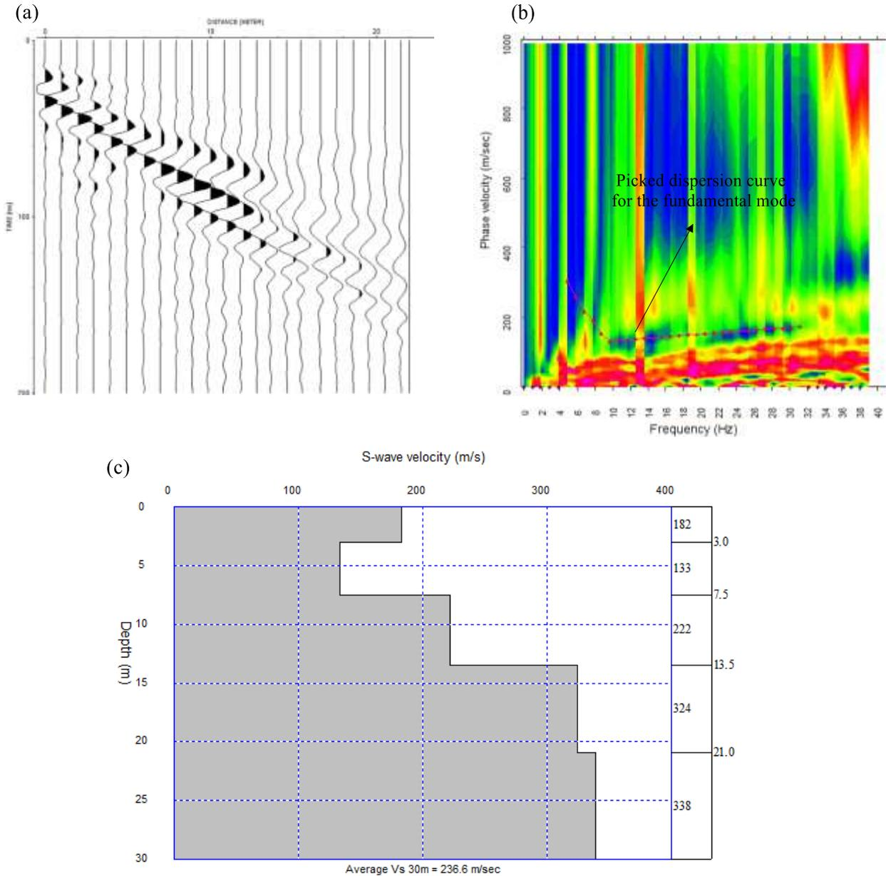
Fig. 7: Profile D-D<sup>1</sup>, A shot gather analysis. (a) 24-channel shot gathers recorded using 10-Hz vertical component geophones. (b) Dispersion spectrum (c) 1D S-wave velocity model estimated by inversion of the dispersion curves picked in (b)
