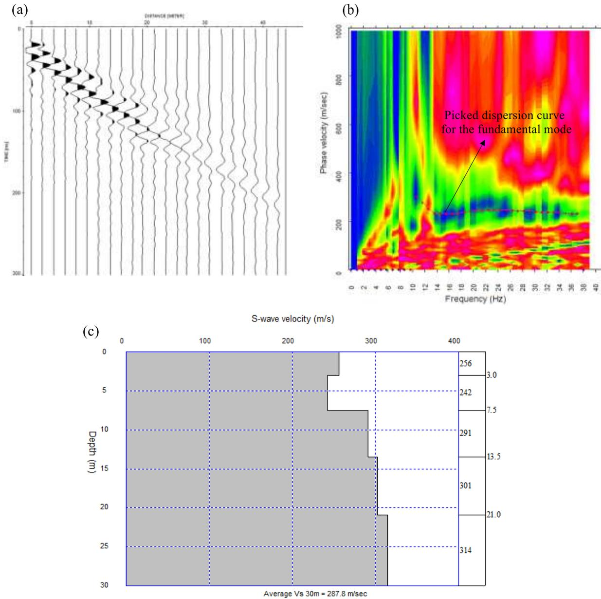
Fig. 6: Profile C-C<sup>1</sup>, A shot gather analysis. (a) 24-channel shot gathers recorded using 10-Hz vertical component geophones. (b) Dispersion spectrum (c) 1D S-wave velocity model estimated by inversion of the dispersion curves picked in (b)
