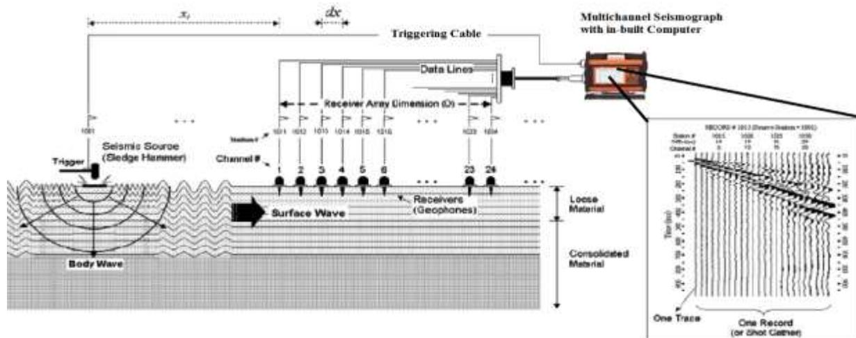
Fig. 2: Schematic illustration for the 1D Multichannel Analysis of Surface Waves (MASW) data acquisition.
