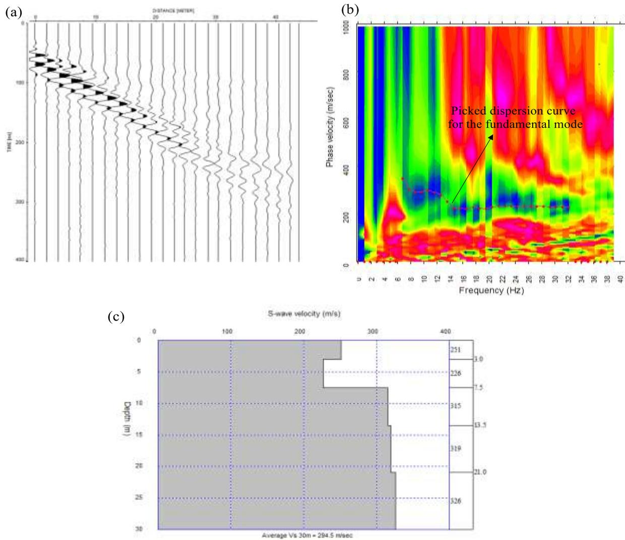
Fig. 5: Profile B-B<sup>1</sup>, A shot gather analysis. (a) 24-channel shot gathers recorded using 10-Hz vertical component geophones. (b) Dispersion spectrum. (c) 1D S-wave velocity model estimated by inversion of the dispersion curves picked in (b)
