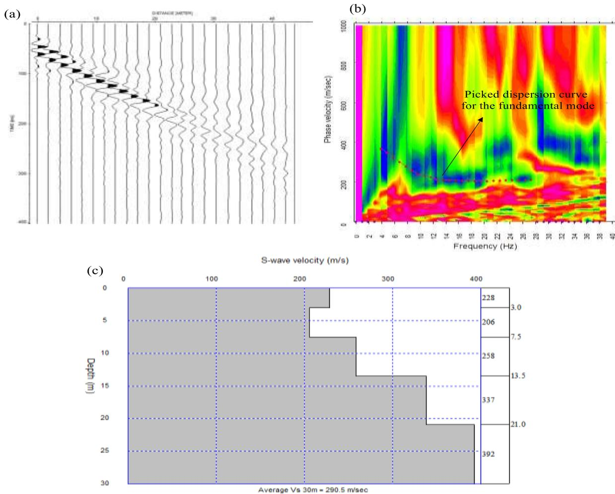
Fig. 4: Profile A-A<sup>1</sup>, A shot gather analysis. (a) 24-channel shot gathers recorded using 10-Hz vertical component geophones. (b) Dispersion spectrum (c) 1D S-wave velocity model estimated by inversion of the dispersion curves picked in (b)
