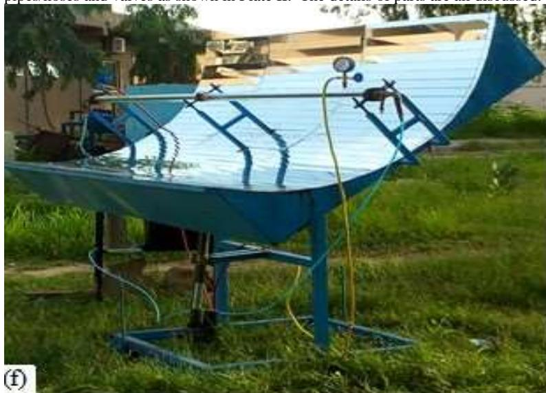
Plate II: Parabolic trough solar collector
