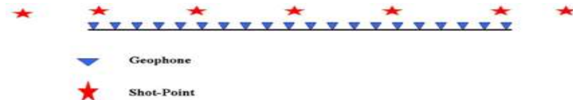
Fig. 2: Profile layout of both P- and S-wave.
