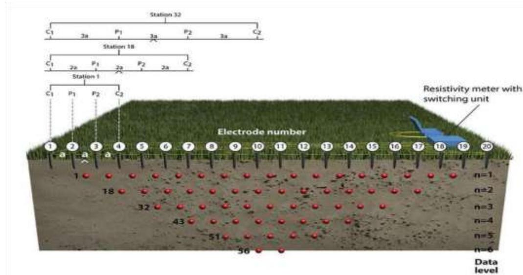
Fig. 3: 2D data collection using multi-electrode resistivity system (Loke *et al.*, 2013).
