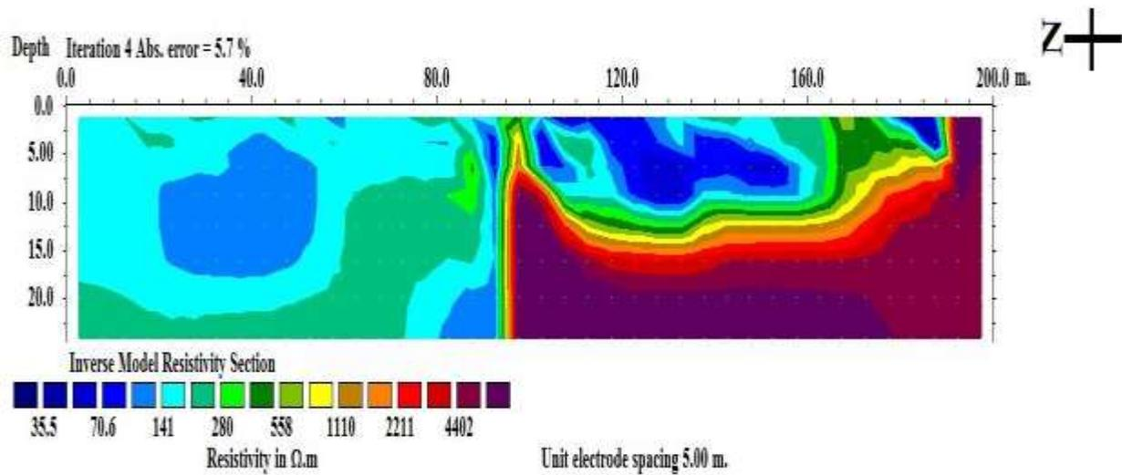
Fig. 5: 2D resistivity inversion model section for profile 2
