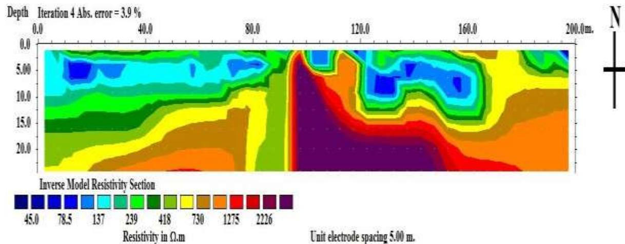
Fig. 4: 2D resistivity inversion model section for profile 1
