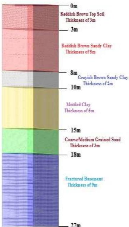
Fig. 7: 3D Geological borehole log used for calibration of the resistivity models
