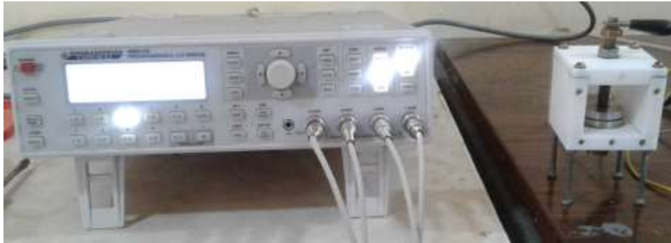
Fig. 1: LCR meter and a test cell
