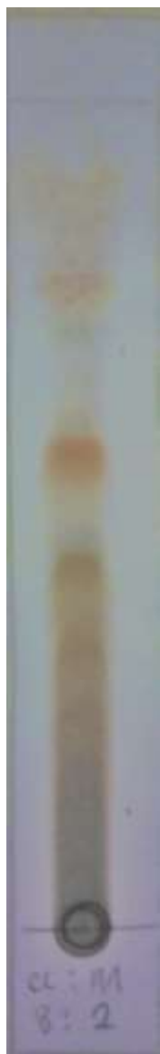
Plate 1: Chromatogram of n-butanol Fraction of Methanolic Extract of M. balsamina in Chloroform-Methanol (8:2) detected with p-anisaldehyde in H_2SO_4
