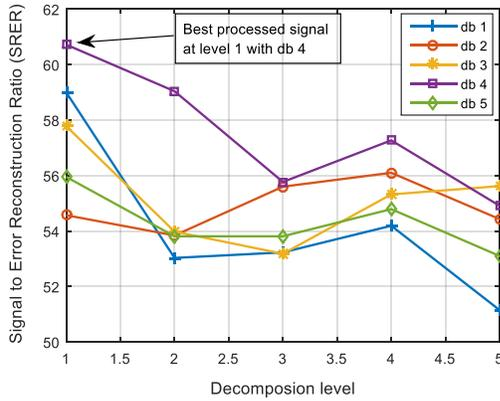
Fig. 8: Processed signals using dB wavelet under soft thresholding.
