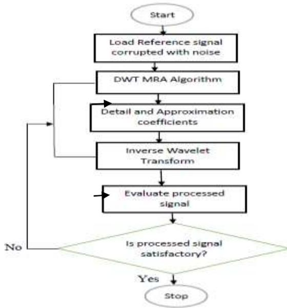
Fig. 2: Block diagram for the Enhanced for the Signal data denoising with WDT
