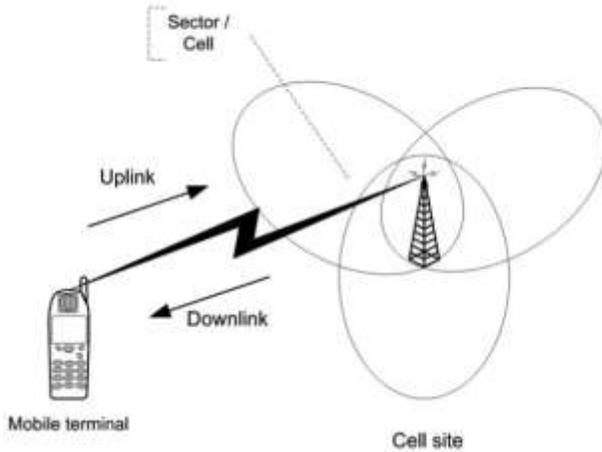
Fig. 1: Mobile Terminal Transmitting Configuration during Field Drive Test
