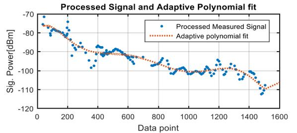
Fig. 10: Best Adaptive Polynomial Fit at Decomposition Level 2 for Sym 4 wavelet family with Hard Thresholding
