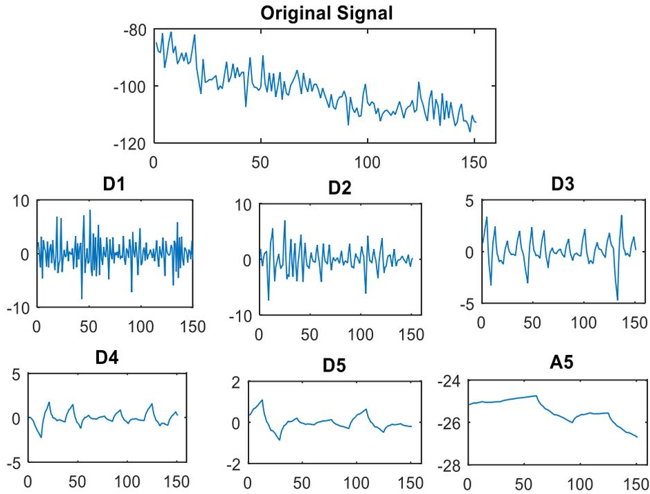
Fig. 5: level decomposition with db2 wavelet
