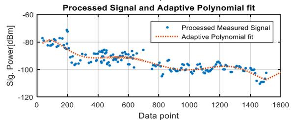
Fig. 11: Best Adaptive Polynomial Fit at Decomposition Level 1 for db 4 wavelet family with Hard Thresholding
