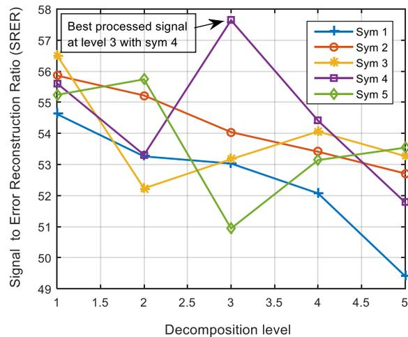
Fig. 7: Processed signals using Symlet wavelet under hard thresholding
