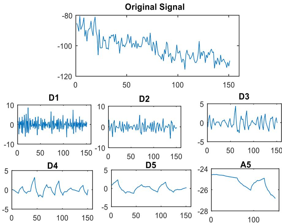
Fig. 4: level decomposition with sym2 wavelet
