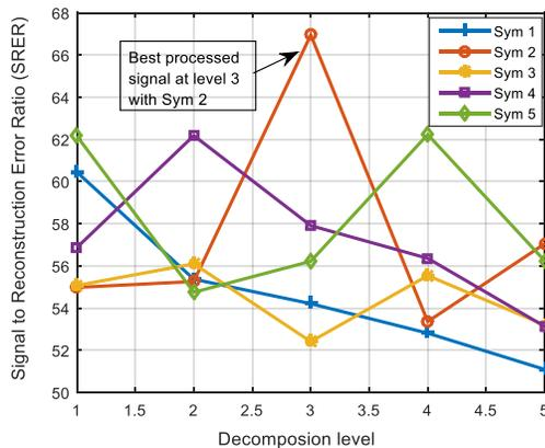
Fig. 6: Processed signals using Symlet wavelet under soft thresholding
