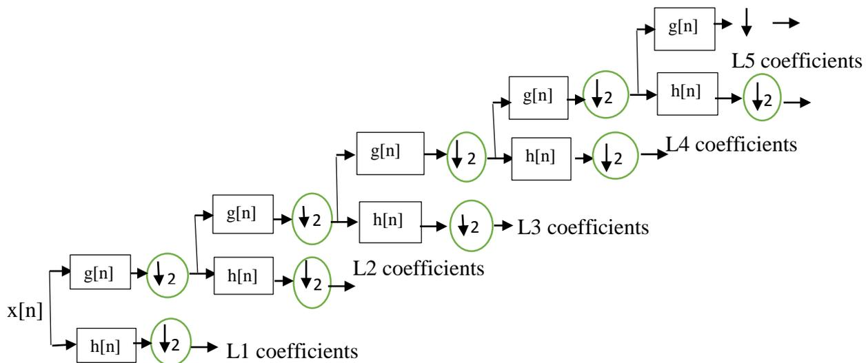
Fig. 3: A Filter bank illustration of different level Decomposition with DWT
