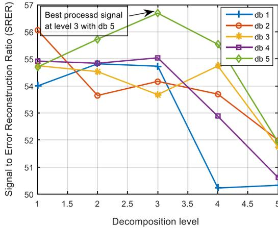
Fig. 9: Processed signals using db wavelet under hard thresholding
