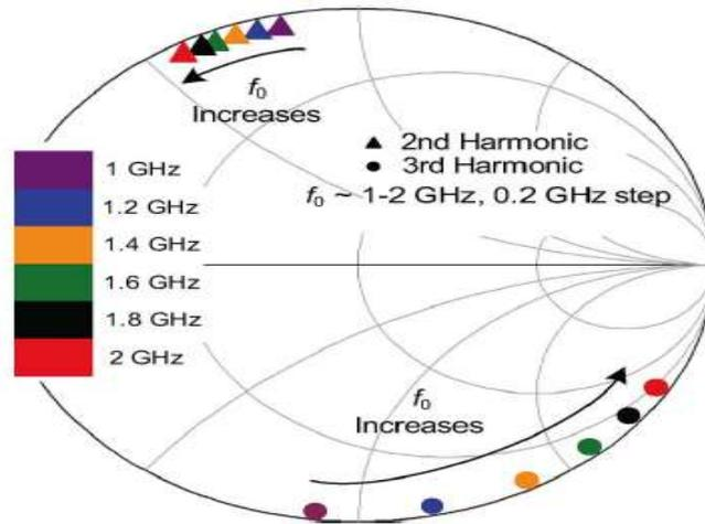
Fig. 3: Optimal impedance of the second and third harmonics
