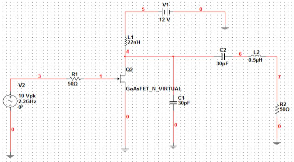
Fig. 1: Configuration of Class-E Power Amplifier
