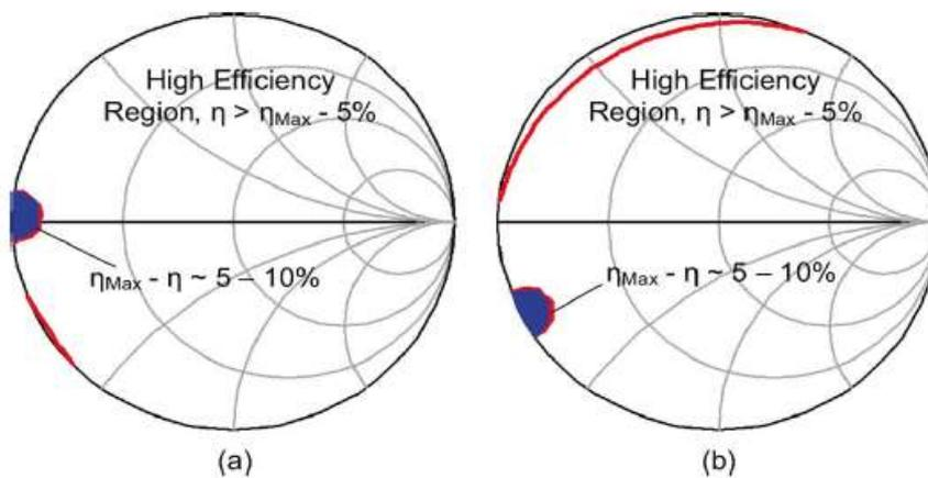
Fig. 5: Simulated load-pull contours of the second harmonic impedance: (a) at  $2f_0 = 3\text{GHz}$  and (b) at  $2f_0 = 6\text{GHz}$ .
