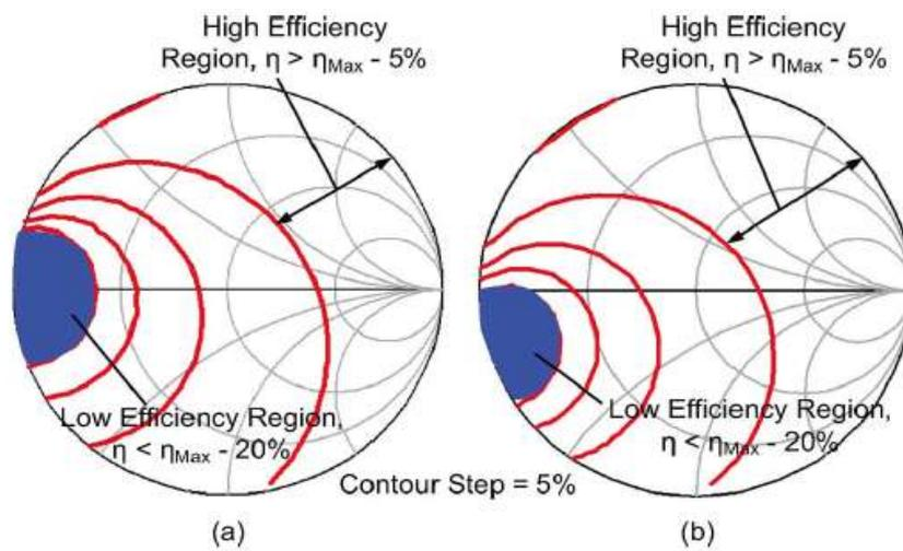
Fig. 4: Simulated load-pull contours of the second harmonic impedance: (a) at  $2f_0 = 2\text{GHz}$  and (b) at  $2f_0 = 4\text{GHz}$ .
