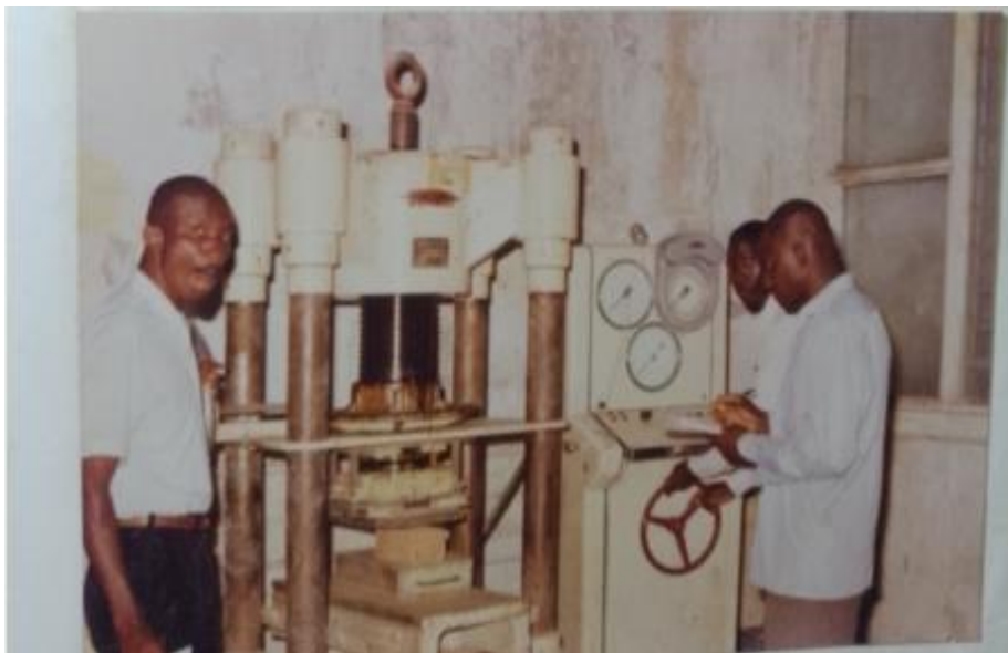
Figure 1: Avery Denison Universal Testing Machine for Strength Determination of Soil Blocks
